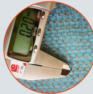
Wire thickness test
