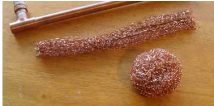
Mechanical part cleaning with copper scrubber
